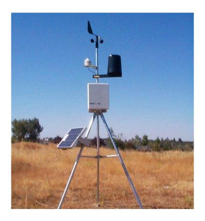
Our Weather Monitoring Station (WMS) automatically monitors site meteorological conditions and photovoltaic panel temperature in real-time, transmitting sensor's data to the Logics PowerAMR IoT based monitoring platform.
